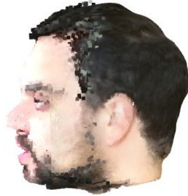
Fig. 6. Reconstructed volumetric video frame from single RGB-D sensor where it’s possible to notice blending artifacts.
