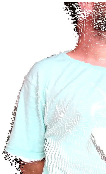
Figure 4.2: RGB-D frame viewed as a point-cloud where a border artifact caused by Kinect's RGB and depth misalignment.
