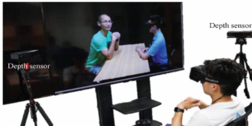
Figure 1.2: User with a Oculus Rift VR glass interacting with another user, while being captured by a setup of three (one hidden) RGB + Depth Microsoft Kinect sensors. A synthesized scene with the two users is shown in the TV in the back.
