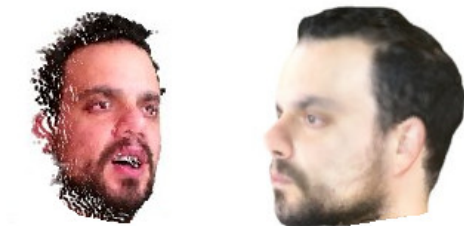
Figure 3.8: Point-cloud view of a RGB-D frame (left) and volumetric model of human head (right).
