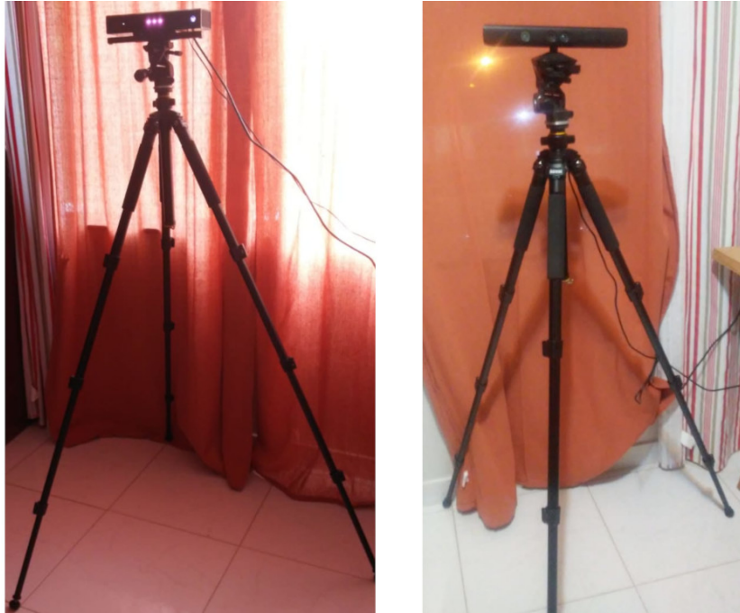
Figure 2.2: Kinect 2 (left) and Kinect 1 (right) assembled on a tripod, in the configuration used in the capture experiments.
