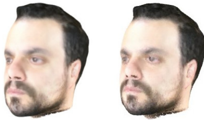
Figure 3.12: Point-cloud before compression (left) and the resulting point-cloud after compression and decompression (right).
