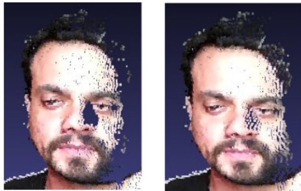
Figure 3.6: A point-cloud created from a single RGB-D frame (left), and the same frame after applied the proposed hole filling algorithm (right).
