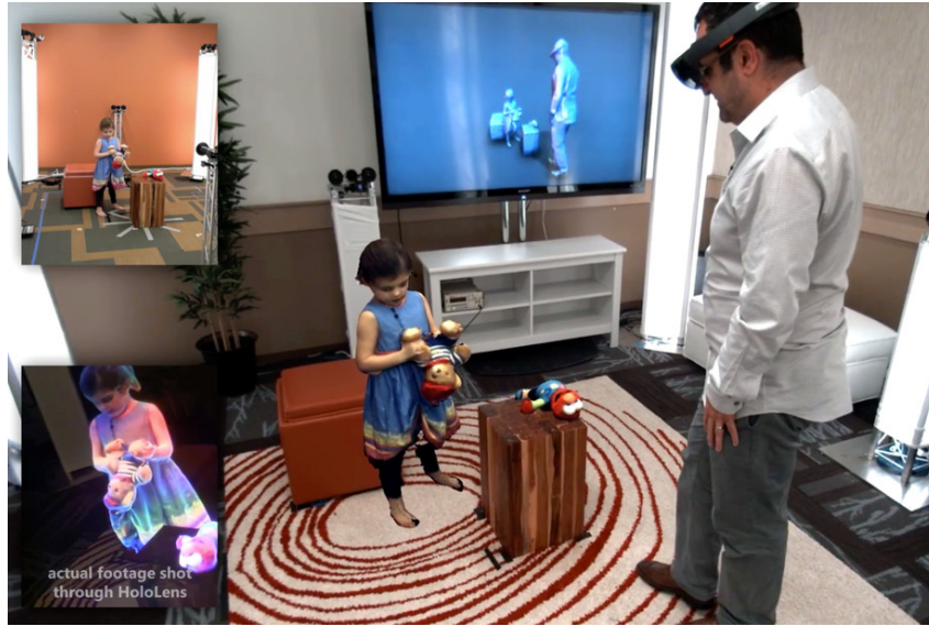
Figure 1.3: User viewing a remote located kid though a MR device. Top left shows the real scene and bottom left the way the scene is viewed in the Microsoft's MR HMD, called HoloLens.
