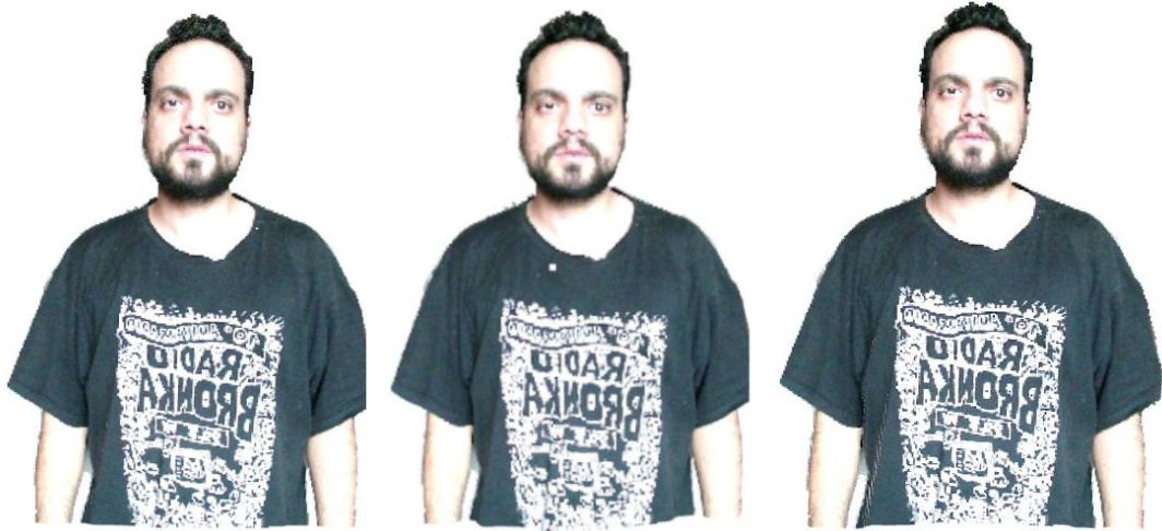
Figure 3.3: Point-cloud created from the original RGB-D frame (left), a point-cloud created with a hole in the depth map in the region of the t-shirt (center) and the view of the point-cloud (right) after the application of the proposed algorithm to the frame with hole (right).
