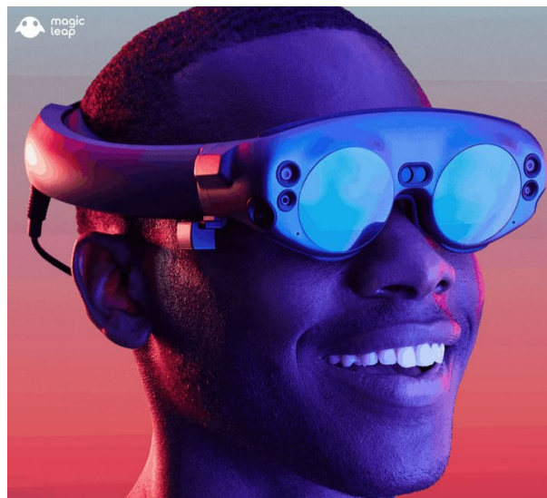
Figure 1.4: Magic Leap One mixed reality head-mounted device. In the image it's possible to see some of the many sensors the device has, including depth sensor.
