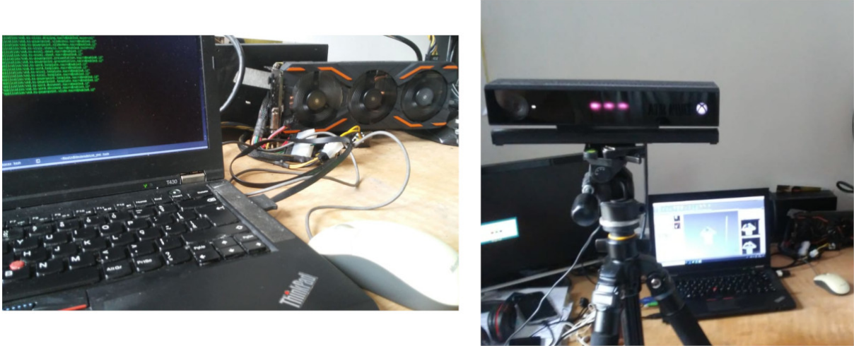
Figure 3.1: Partial view of the notebook with an external GPU attached (left) and the Kinect 2 connected to the notebook computer used for capture outside the laboratory (right).
